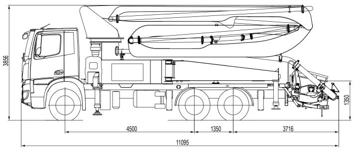
Note: Dimensions varing according to truck assembly (mm). For illustration only
