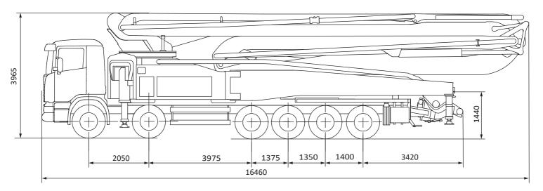
Note: Dimensions varing according to truck assembly (mm). For illustration only
